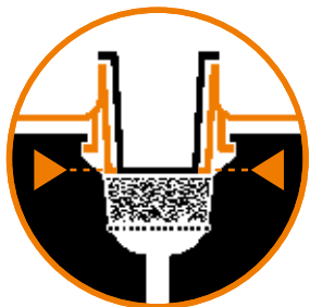
The lower rim of the Filling Aid must be above the top level of the plant material
