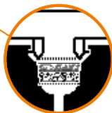
Filling Chamber partially filled, with Liquid Pad placed on top
