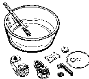
Manual cleaning of the disassembled Cooling Unit
