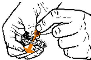
Removal of the large Base Seal Ring
